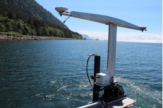
Universal Sonar Mount Designed for Applanix Pos MV & R2Sonic 2022 /2024/2026
